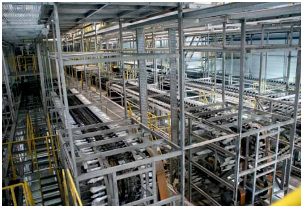
Modern immersion facility for glove manufacturing in Surat Thani, Thailand
